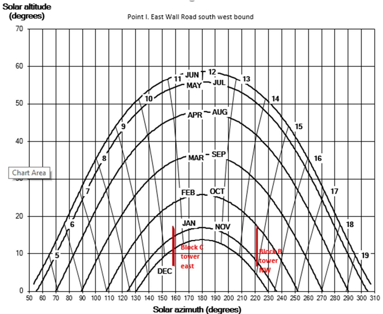
Figure 12. Sunpath diagram showing times of day and year for which sunlight can be reflected to point I.
