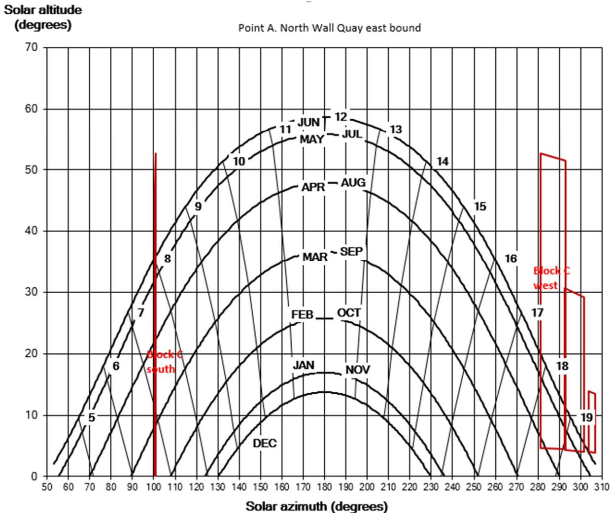
Figure 3. Sunpath diagram showing times of day and year for which sunlight can be reflected to point A.
