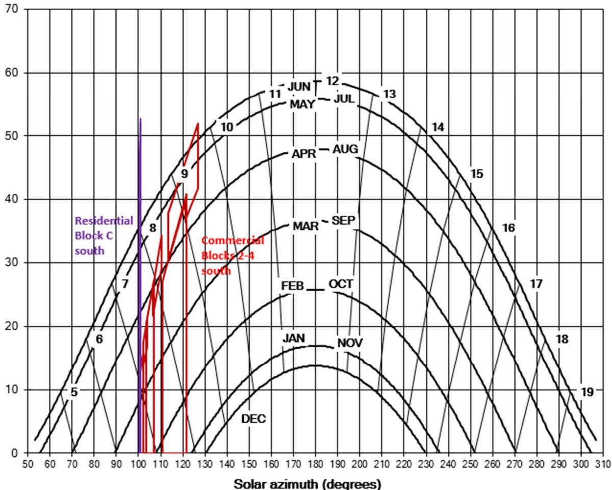
Figure 16. Sunpath diagram showing times of day and year for which sunlight can be reflected to point A (both schemes together).
