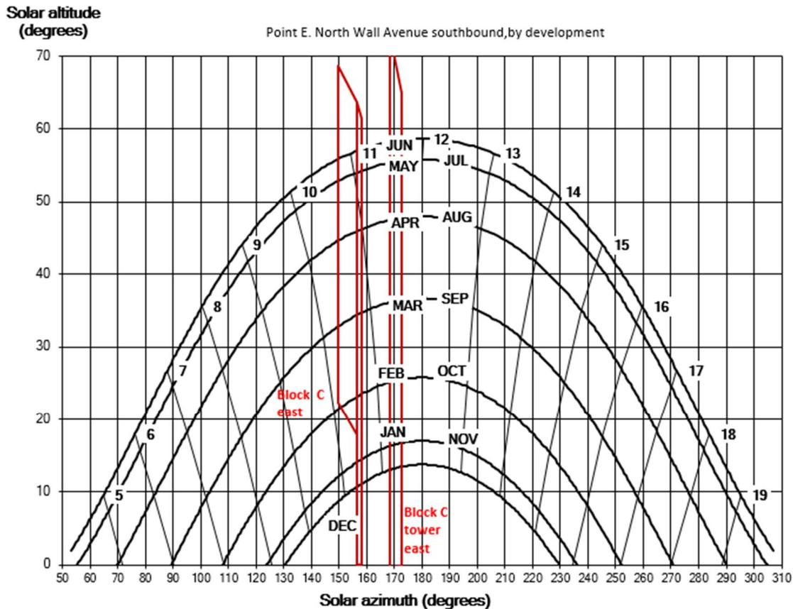
Figure 8. Sunpath diagram showing times of day and year for which sunlight can be reflected to point E.
