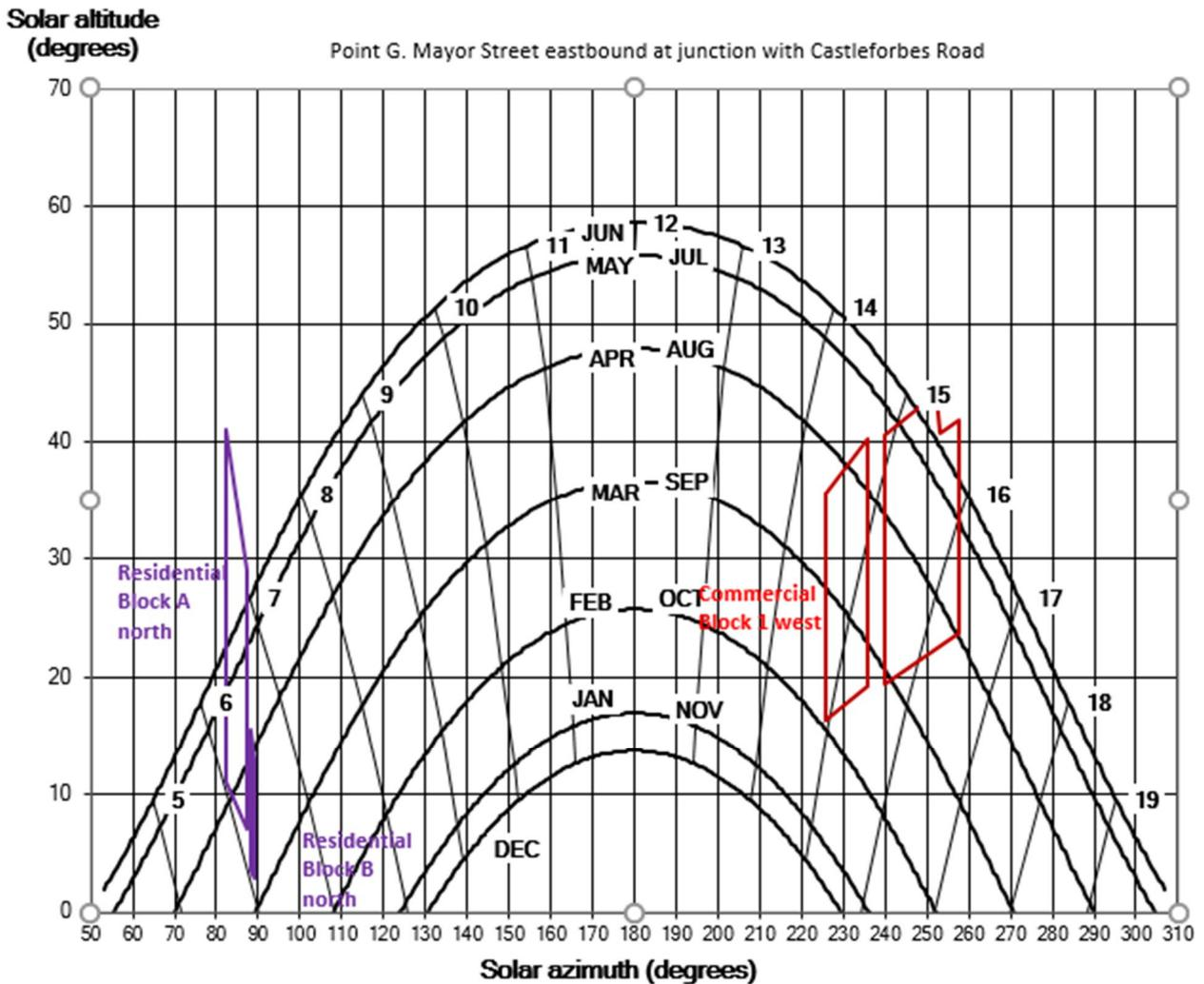
Figure 18. Sunpath diagram showing times of day and year for which sunlight can be reflected to point G.
