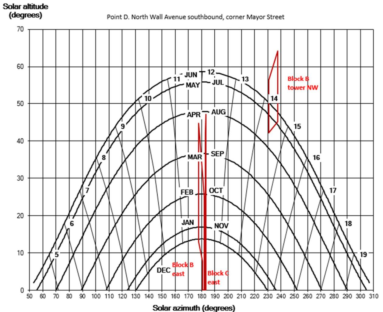
Figure 7. Sunpath diagram showing times of day and year for which sunlight can be reflected to point D.
