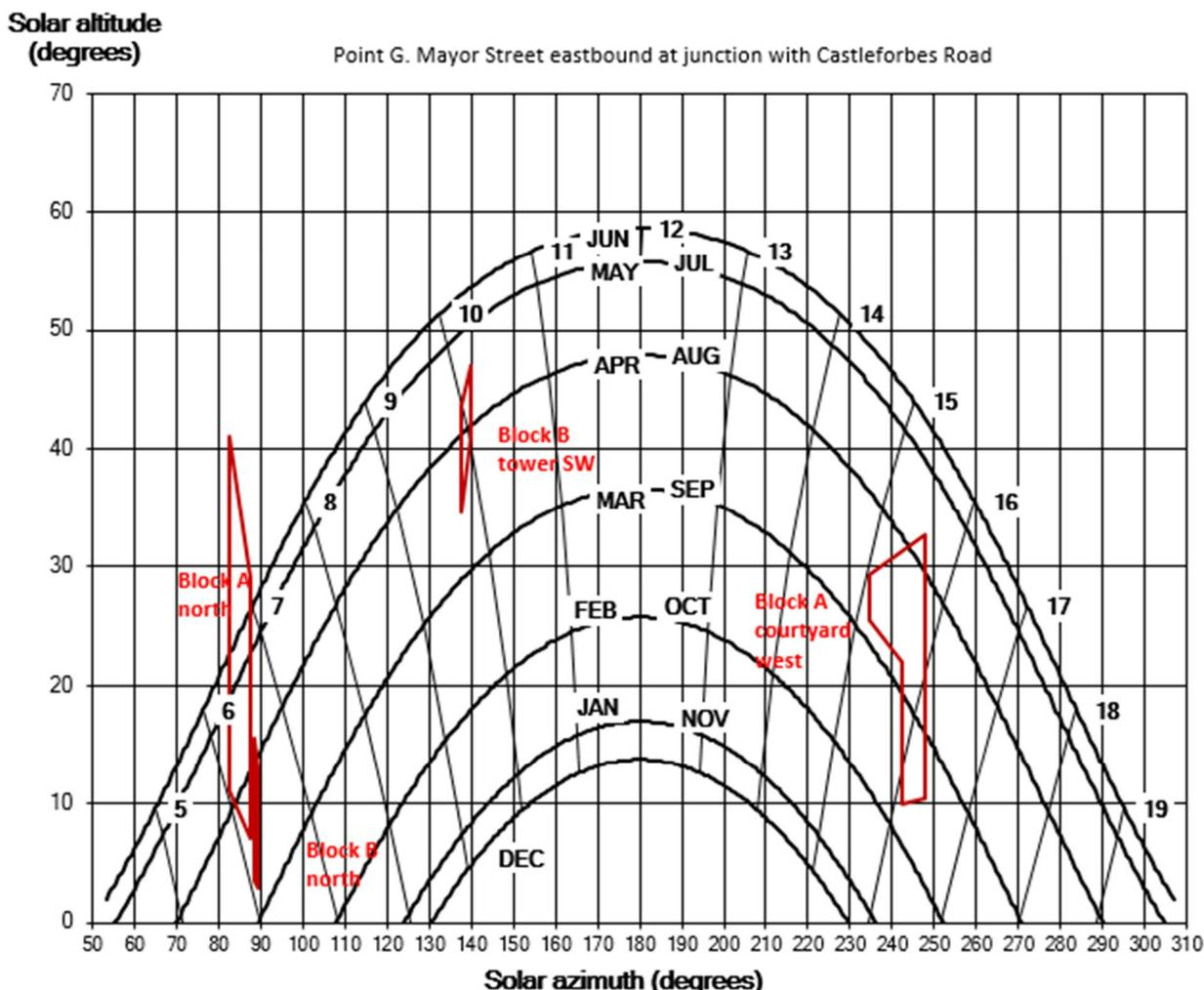
Figure 10. Sunpath diagram showing times of day and year for which sunlight can be reflected to point G.
