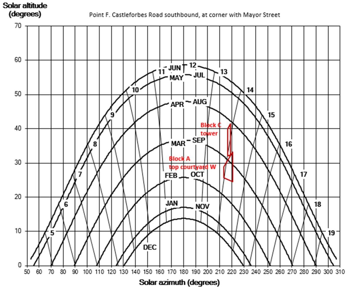
Figure 9. Sunpath diagram showing times of day and year for which sunlight can be reflected to point F.
