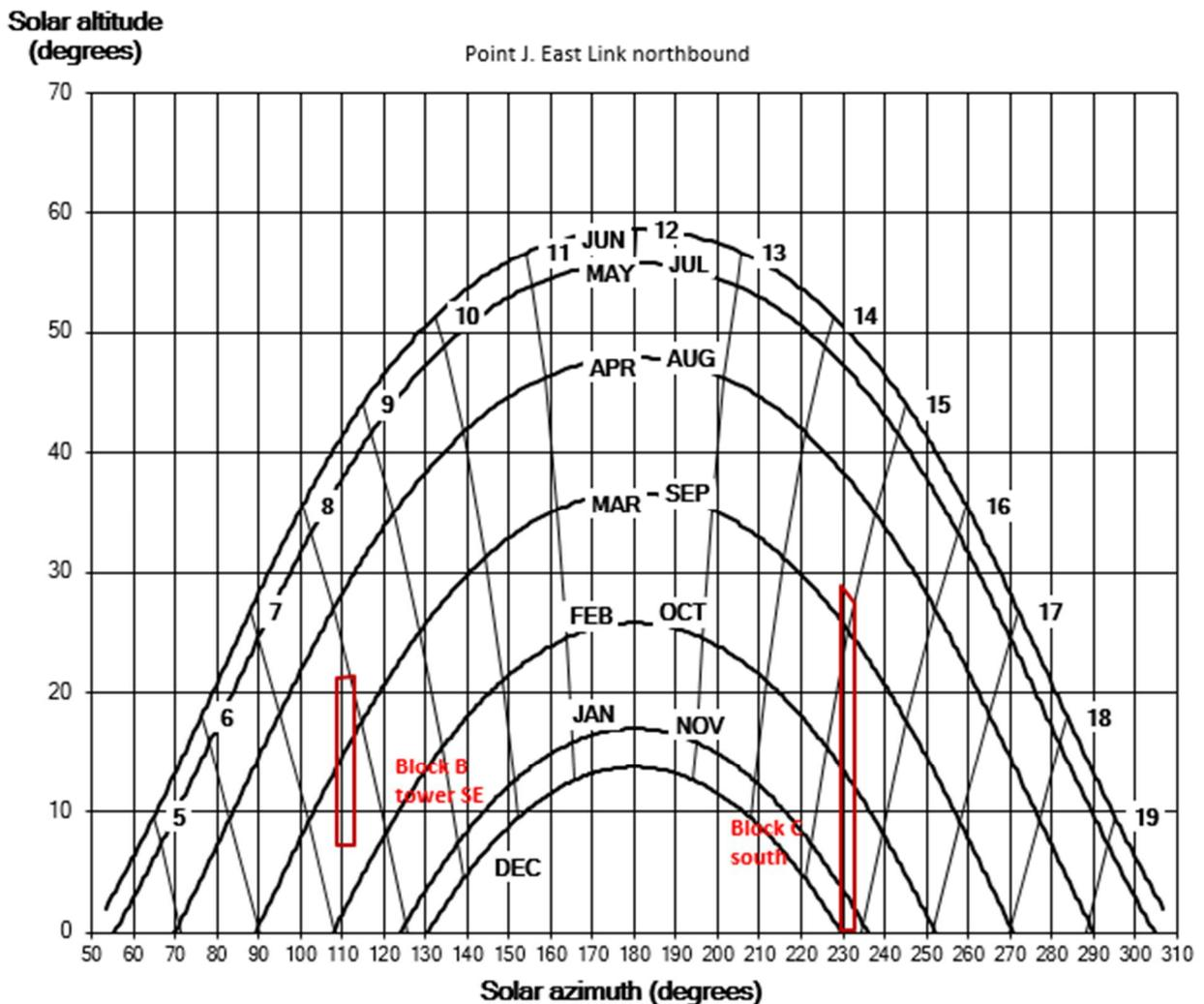
Figure 13. Sunpath diagram showing times of day and year for which sunlight can be reflected to point J.
