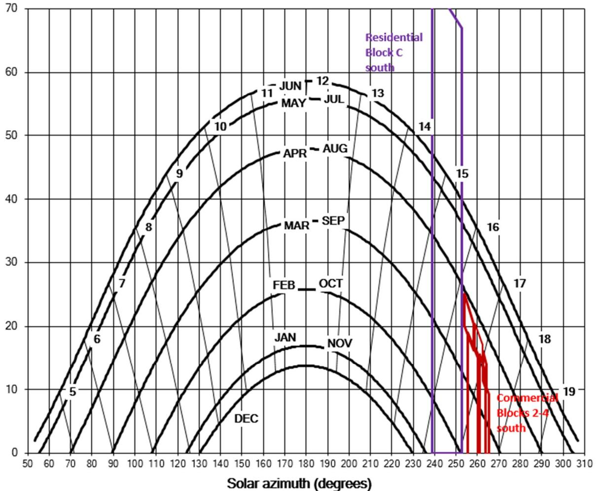
Figure 17. Sunpath diagram showing times of day and year for which sunlight can be reflected to point B (both schemes together).
