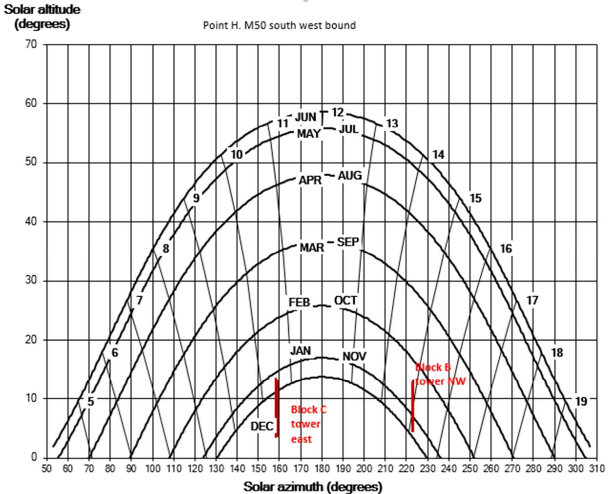
Figure 11. Sunpath diagram showing times of day and year for which sunlight can be reflected to point H.
