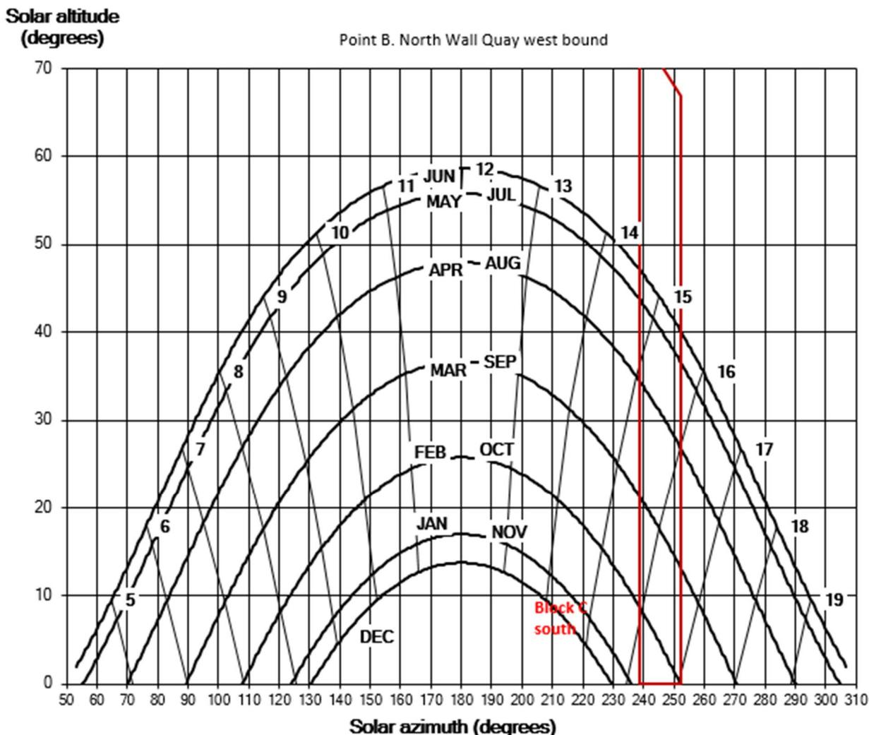
Figure 4. Sunpath diagram showing times of day and year for which sunlight can be reflected to point B.
