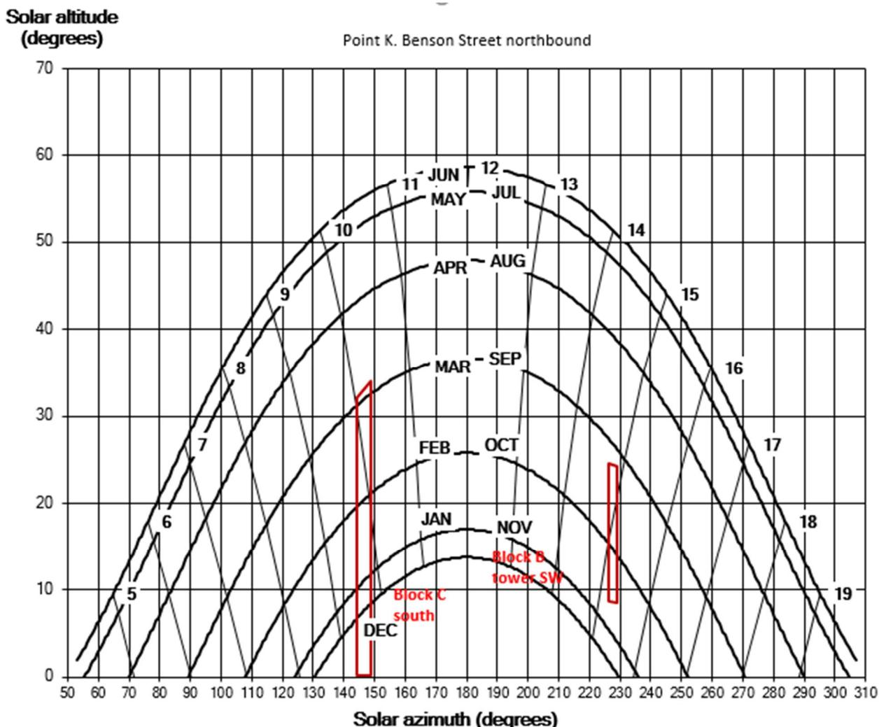
Figure 14. Sunpath diagram showing times of day and year for which sunlight can be reflected to point K.
