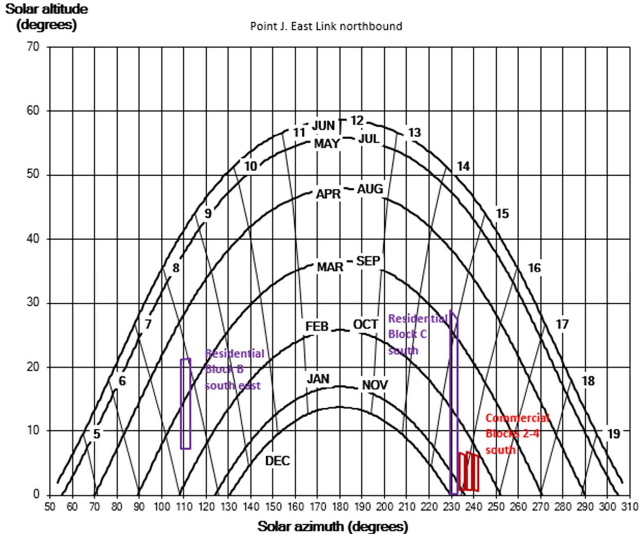
Figure 19. Sunpath diagram showing times of day and year for which sunlight can be reflected to point J.
