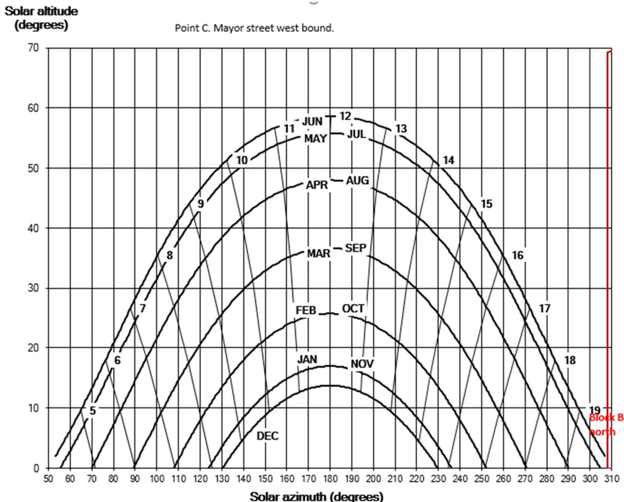
Figure 6. Sunpath diagram showing times of day and year for which sunlight can be reflected to point C.
